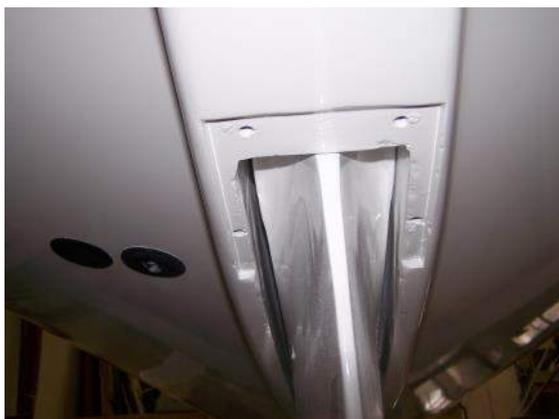
Left: Rear of keel showing mounting holes for bolts. These need to be well sealed with a suitable sealant...
