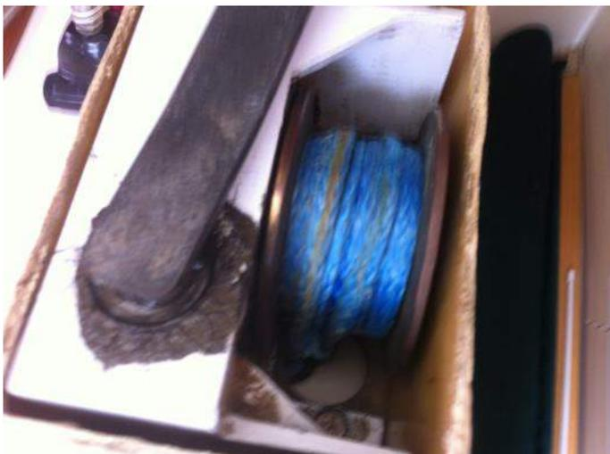
age, possible keel loss, and a lot of frustration and heartache! Also, I have now attached a piece of string to the keel locking pin with a loop at the end. Once I have inserted the pin, I loop the end over the keel winch handle to serve as a reminder. Lastly, it is probably a good idea to have a few bits 'n pieces and tools on the boat specifically for this eventuality.
