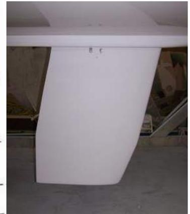
Keel fully extended showing pins...
